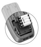
3 Plug the cable of the battery pack in the connector.
